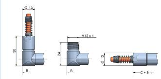
Sensors with cable output have a cable fitting and a spring for bend protection of the cable. For installation, the bending radius should not be less than 3 times the cable diameter. The standard cable length is 2 m.
