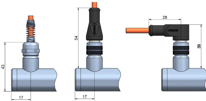
Sensors with cable output have a cable fitting and a spring for bend protection of the cable. The standard cable length is 2 m.
