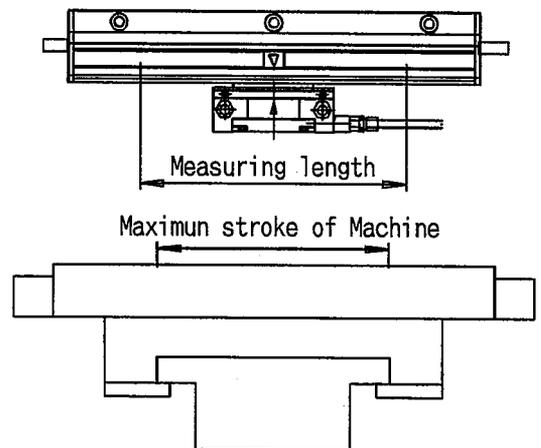
The scale will be damaged if it moves beyond the measuring length.
