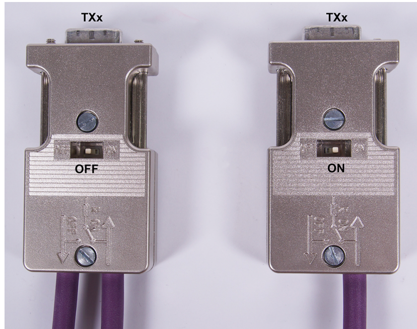
Figure 1: CAN-Bus connectors with integrated termination.
