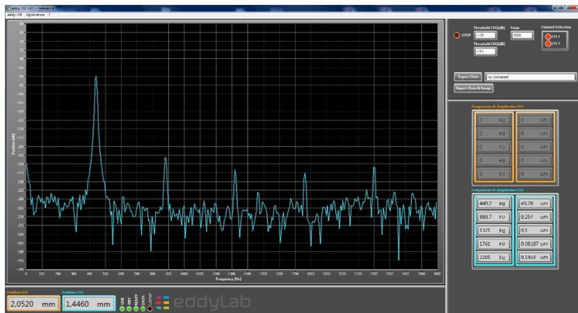
Figure 4: FFT of a tuning-fork.
