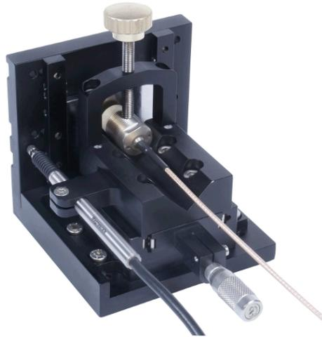
Figure 9: Portable linear stage with a linear encoder (Magnescale) - eddy current sensor and a target with the dimensions  $50 \times 50 \times 5 \text{ mm}$ .
